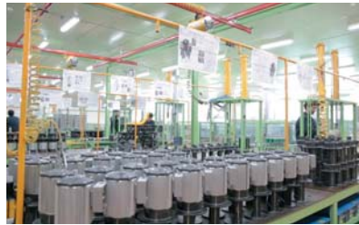
▲Coolant pump 조립 Line
